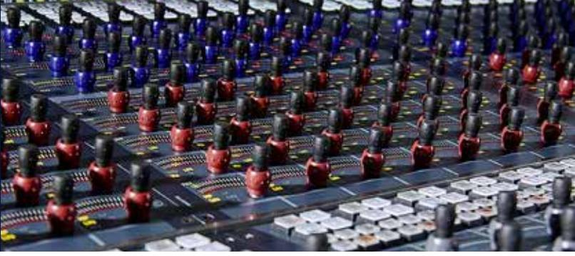
twist is the key action: When pressed shortly, it toggles PFL ON/OFF. Pressing and holding it will allow for momentary monitoring. Combined with the option to also use the lower fader stop for switching PFL, which generally works in summing mode, the engineer always has all options at hand without the need to switch functionalities in the Master section.
